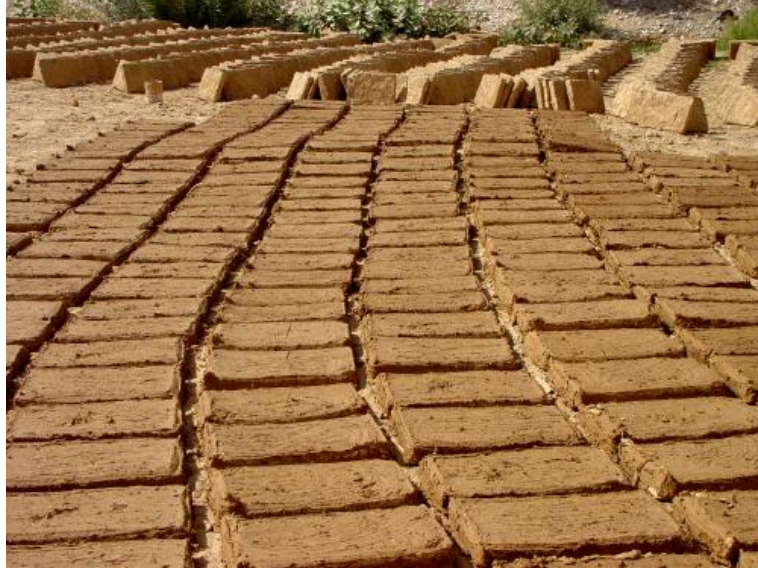
Figure 3: Sun dried adobe blocks: Source: http://buildinglocal.files.wordpress.com/2011/10/adobe-2.jpg
